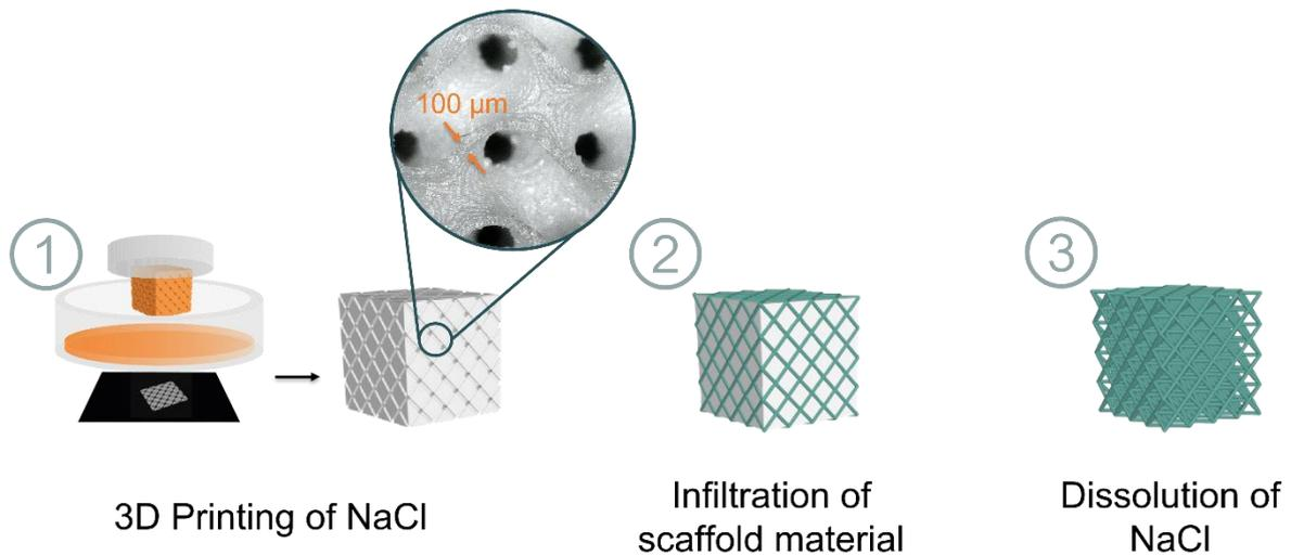
Figure 1 sallea's process to manufacture 3D cell scaffolds.
